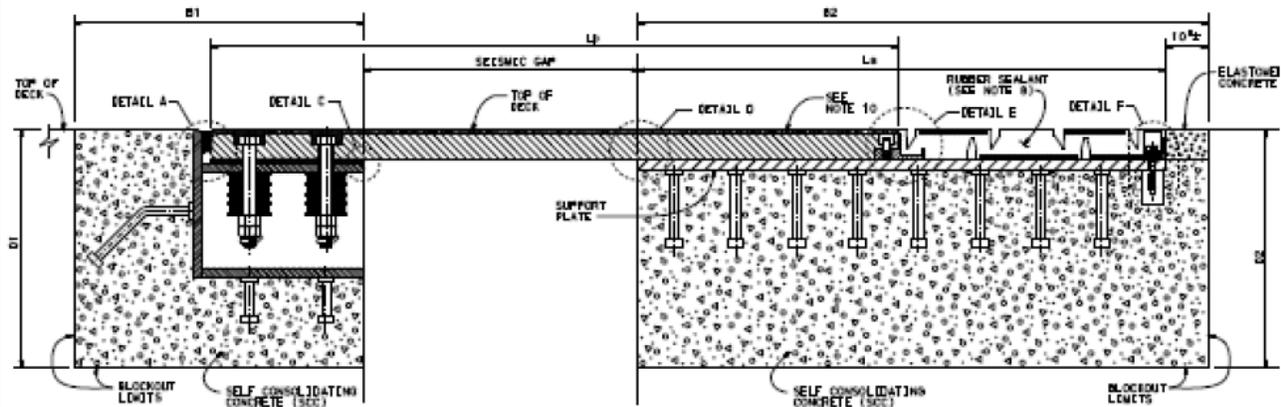
Figure 2.4-36. California Plate Joint Seal Assembly (Type II). Isometric and Section
